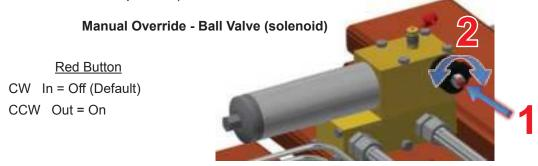
**NOTE:** The floor can be stopped by returning the red handle or red button to the original position.
